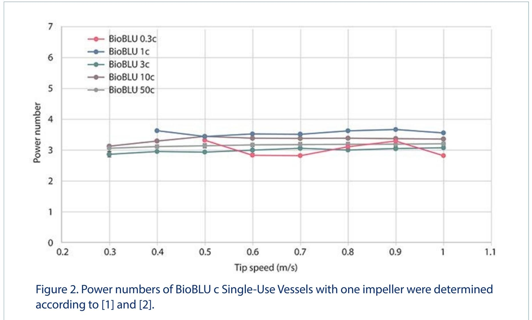
Figure 2. Power numbers of BioBLU c Single-Use Vessels with one impeller were determined according to [1] and [2].
