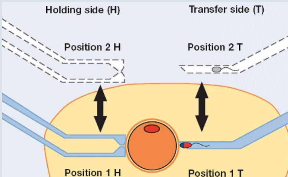
Electronic capillary position storage of the TransferMan 4m also enables fast switch between positions in and above the medium droplet – for fast change between droplets, increased working speed, and higher survival rates.
