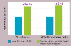
\*Data represents the mean of three flasks/plates, setpoints:  $37^{\circ}$ C, 5 % CO<sub>2</sub>, 125 rpm, rh for device with steam humidification set to 85% (max)
