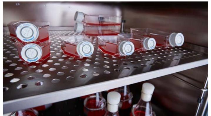
Removable shelf enables shaking of suspension cell cultures while incubating adherent cells under the same conditions
