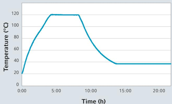
The HTD feature heats the internal chamber to 120 °C and holds it for 4 hours to effectively eliminate contaminants
