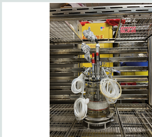
Figure 10: Completed vessel assembly ready for autoclaving.
