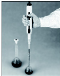
Fig. 4-6: Aspirating the liquid
