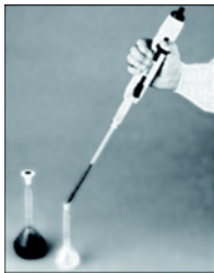
Fig. 4-7: Dispensing the liquid
