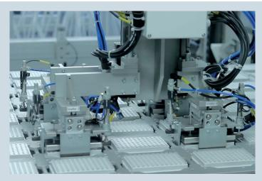
Manufacturing is done under clean room conditions and is a fully automated process eliminating human interaction as much as possible.
