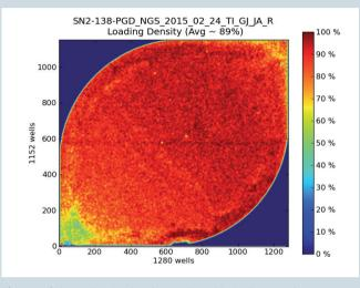
Figure 2: Chip loading density after loading with the Eppendorf Xplorer plus electonic pipette. Loading density was ~89 %.
