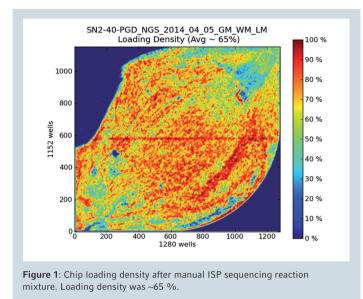
Another parameter relevant to the method's evaluation is the reproducibility of the loading level. During the operators' manual pipette handling, the coefficient of variability was reaching more than 24 %, making it difficult to ensure efficient loading level in every run. Switching to the electronic The chips' ISP loading value is calculated by the sequencer and loading density is displayed in a graphic manner (fig. 1 and 2).
