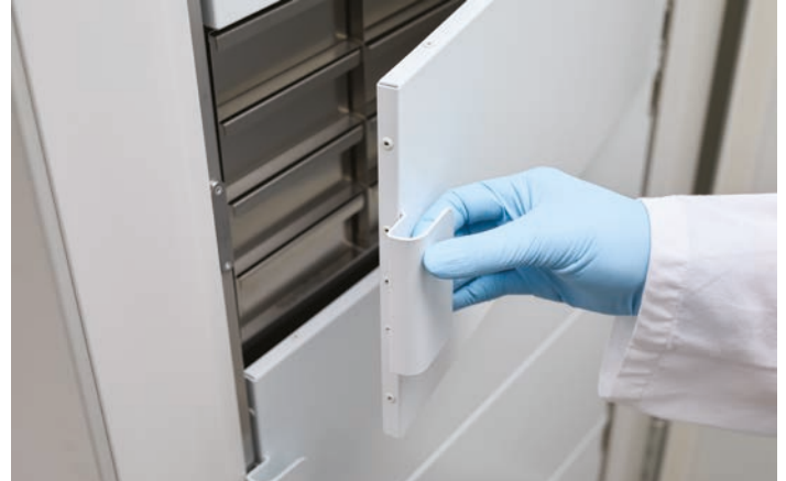
Figure 6: Every door opening of an ULT freezer results in a warm-up of the inner compartment which requires a fast pull-down back to the setpoint
