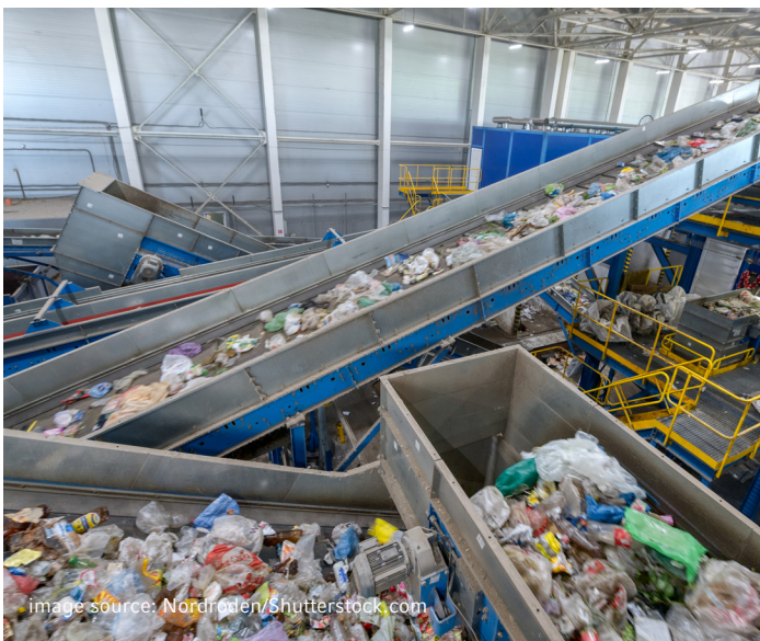
Automated sorting process for used plastic material
