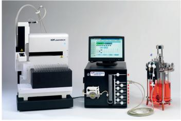
Fig. 2: Seg-Flow 4800 Automated On-line Sampling System with FlowFraction™ 400 Fraction Collector
