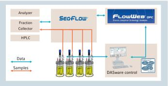
**Fig. 3**: Architecture for the Seg-Flow 4800 process trigger sampling function. The process event or "trigger" is user-defined and is programmed in the bioreactor's OPC-enabled SCADA or bioprocess management system, which remotely controls the Seg-Flow system.
