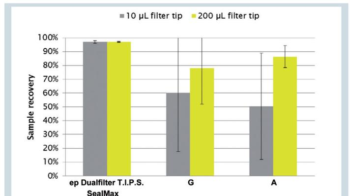
**Figure 3:** Comparison of sample water recovery rate between different manufacturers of self-sealing filter tips. Values presented are average percentage of sample recovery calculated from 10 individual measurements. The error bar represents standard deviation.
