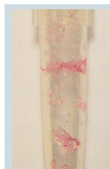
**Figure 4:** Sample liquid became slightly viscous and had tendency of foam formation after coming into contact with the filter (filter tip from one of the two other manufacturers tested). This observation was made during the investigation, in which distilled water (colorless) was used as test liquid. For visualization, the picture shows test using distilled water with added red dye.
