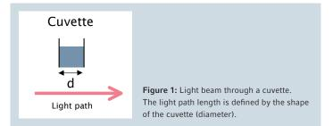
If a microvolume plate such as the Eppendorf  $\mu$ Plate G0.5 is used, the distance between the upper and the lower side of the plate (or the quartz wells, respectively) will determine the path length. In the case of the Eppendorf  $\mu$ Plate G0.5 this distance, and therefore the path length, is 0.5 mm (G = gap 0.5 mm). This feature considerably simplifies concentration determination via extinction factor on the microvolume scale.
