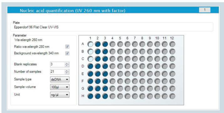
Figure 4: Screenshot of the method "Nucleic Acid quantification (UV 260nm with factor)" from the software of the PlateReader AF2200.
