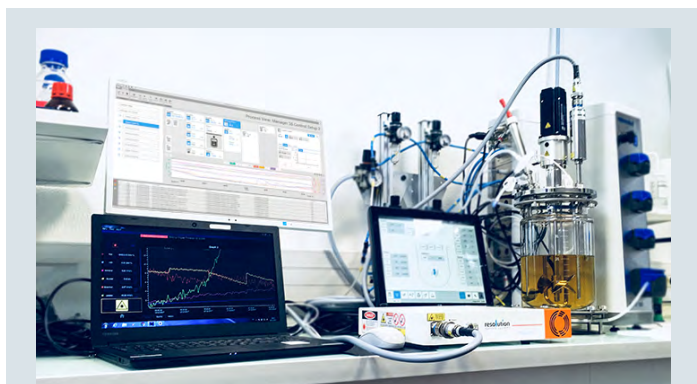
Fig. 1: Illustration of the complete system setup with the ProCellics probe inside the bioreactor controlled by DASware control 5.
