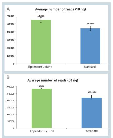
**Figure 2:** The average number of reads of a 10 ng (2 A) and 50 ng (2 B) NGS library prepared from total RNA of primary HUVEC cells in Eppendorf LoBind and standard plates. The average number of reads is up to 23 % higher in Eppendorf LoBind than in standard plates (n=3).
