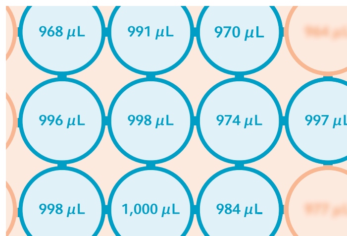
10 measurements – avg. 984 µL, 1.6% error
