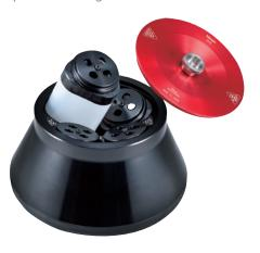
With its compact design, Rotor R9A2 greatly improves harvesting process efficiency through the use of unique 1.5 L triangular wide-mouth bottles. Processing up to four 1.5 L bottles (6 liters) at up to 15,100 x q, this fixed-angle rotor is ideal for harvesting of bacteria, mammalian or insect cells, as well as algae or yeast. By reducing the number of bottles required to spin 6 L from the standard six to just four, processing time can be reduced by up to 32% without impacting pelleting efficacy.
