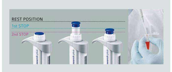
Reverse pipetting shown in 3 steps. The blow-out volume is aspirated additionally and remains in the tip, so that the set volume is delivered accurately.
