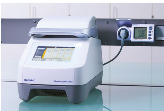
Simple power meters can provide you information which equipment requires the highest amount of energy and where “shut-off” policies may make sense
